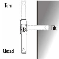
If fitted, turn the key to unlock the window.
